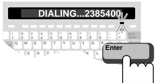
5. When the other TTY starts ringing, the display and Signal light flash slowly and **LINE IS RINGING** is displayed.
